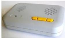
The new **Zavox Reo** is a personal voice amplifier designed to reduce vocal strain and amplify the softest voice. It has been developed especially for clients who have Parkinson's or a condition that makes speaking loudly difficult.
