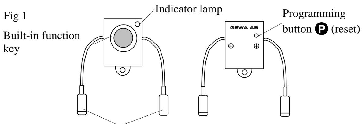
For connection of external control switches with 3.5 mm phone plug
