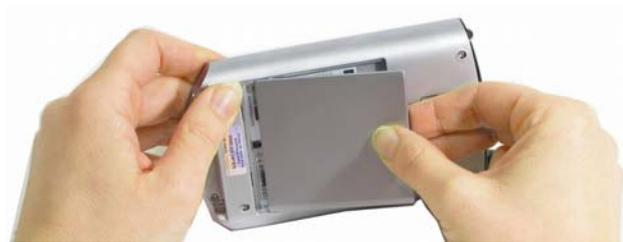
3. Mount the battery into the Pocket-PC again and then insert the Pocket-PC into the Progress Module.
