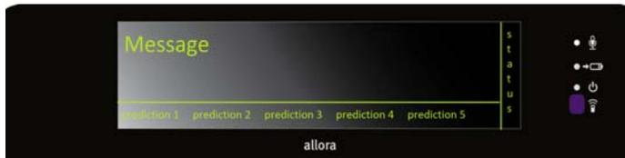
The first screen is divided into three parts. The largest part is used to write the messages. One message can contain multiple lines. If you press the Enter key, the message will be pronounced. You do not have to remove the message to write a new message, which means that you can easily return to your previous
