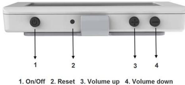
The 2nd display has a number of control buttons. These control buttons only become active when the 2nd display is detached from the main device.
